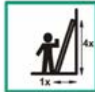
Appropriate ladder adjustment angle
