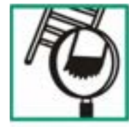
Check ladder footing.
