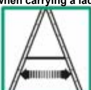
Ensure that the double ladder is always fully extended before use
