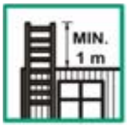
The overlap of the ladder above the point of contact
