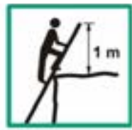
The overlap of the ladder above the point of contact
