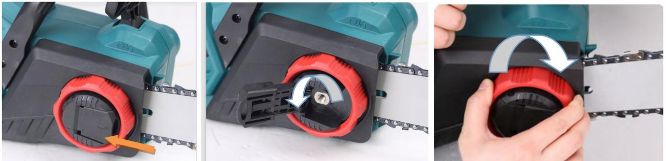
2. Turn the tension knob clockwise to tighten the saw chain until the lower side of the saw chain fits in the guide bar rail as illustrated.
