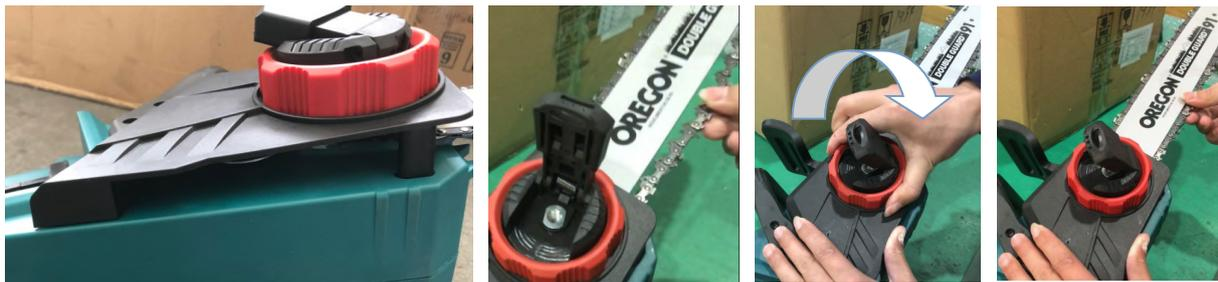
6. Turn the tension knob clockwise and check the chain tension; keep turning clockwise until of suitable tense. To check the suitable saw chain tension, pull the saw chain by the force of about 1kg, if there's distance 5-7mm between the saw chain and guide bar as shown in below, the tension is suitable.
