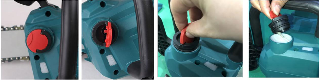
After refilling, hold the chain saw away from the tree. Start it and wait until lubrication on saw chain is adequate.
