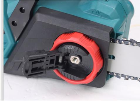
3. Remove the sprocket cover then remove the saw chain and guide bar from the chain saw body.
